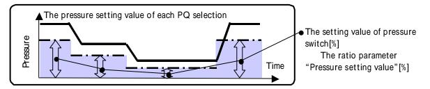
Pressure switch working example
