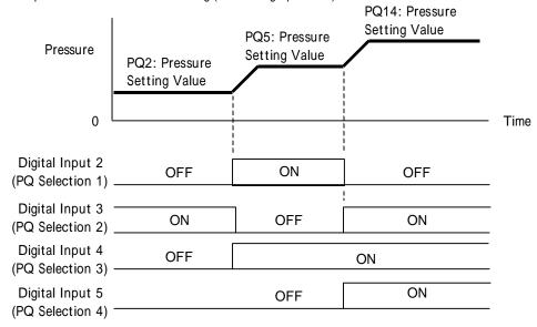
Pressure and flow rate change time when the PQ selection switches
