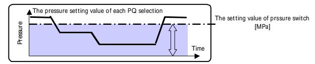
Pressure Unit: the setting value of "P08: Alarm output mix" is "2"  $\,$
