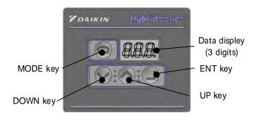
The operation panel is comprised of the 3-digit LED as shown in the left figure. There are four switch keys.
