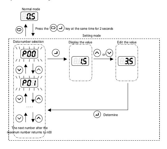
Press the or key to select the displayed data number. Display will flash if the data number is under selection.
