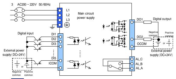
: It is located in the "main power supply terminal" of the controller. Please be sure to wire
