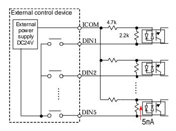
Combination of digital inputs for P-Q selection
