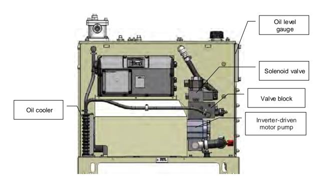
Solenoid valve is not attached to SUT06S3016-30 and SUT06S6007-30.
