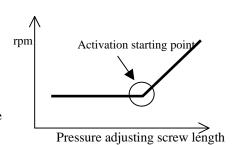
[7] Tighten the lock nut. The safety valve adjustment procedure is completed. (When tightening the lock nut, be careful not to allow the adjusting screw to turn.)
