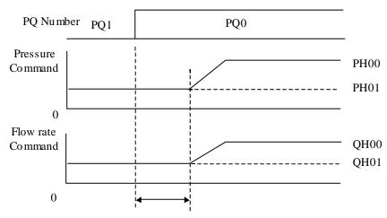
[P12: Solenoid valve response delay time]
