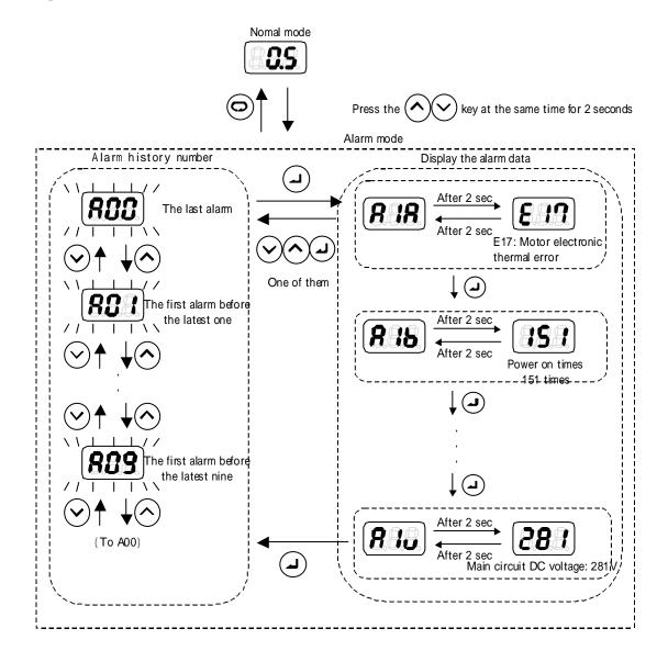
Press the key at the same time in normal mode. It will switch to alarm mode after about 2 seconds.
